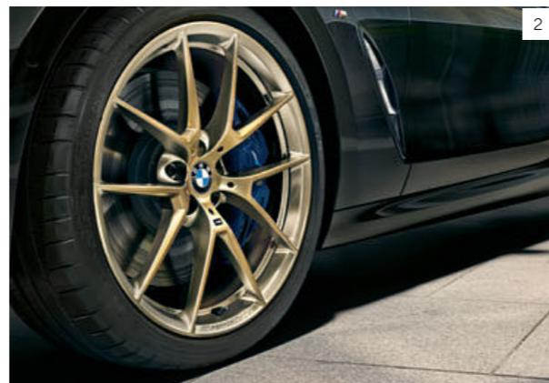
The reverse twist of the filigree Y-spokes ensures maximum lightweight construction. For the unique depth effect, the pigmented, semitransparent base coat is applied to the previously high-gloss polished wheel.
